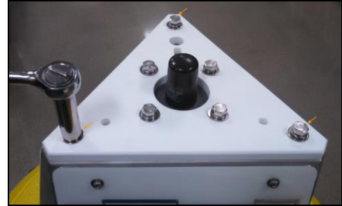
Figure 6: Top Plate Removal
