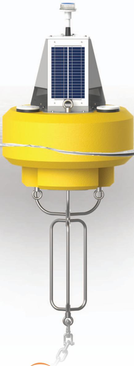
The NexSens **CB-450** Data Buoy is designed for deployment in lakes, rivers, coastal waters, harbors, estuaries and other freshwater or marine environments. The floating platform supports both topside and subsurface environmental monitoring sensors including weather stations, wave sensors, thermistor strings, multi-parameter sondes, Doppler current profilers and other monitoring instruments.
