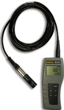
The EC300A is designed for quick, accurate results in an economical platform. The ability to measure conductivity, salinity, TDS and temperature in a simple, compact handheld allows the instrument to be used across multiple application sampling strategies. With a one-year instrument and electrode warranty, waterproof case and ease-of-use, the EC300A will fit your needs.
