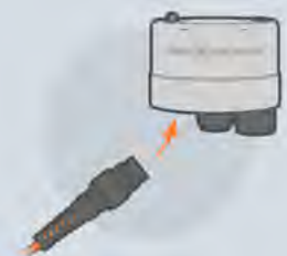
1. Connect Sensors to the Data Logger
