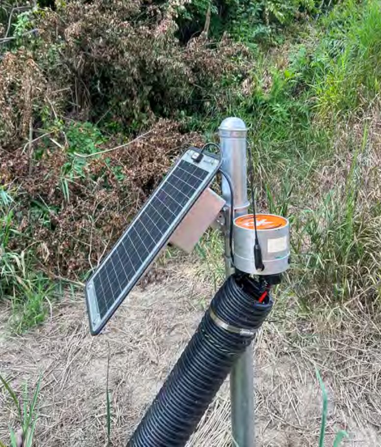
(Top) Upper Scioto River sampling site in Kenton, OH. This site does not have a building, so the X2 data logger and sondes, located down in the river, are powered by the solar panel. (Bottom) Illustrated example of an HTLP Station.
