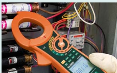
Built-in non-contact Voltage detector with LED alert
