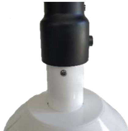
Figure 14: Miniaervane properly installed
