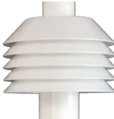
Figure 2: RHT sensor solar shield housing
