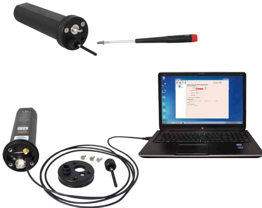
Figure 5-1 Connecting a LevelSender to a computer via USB cable
